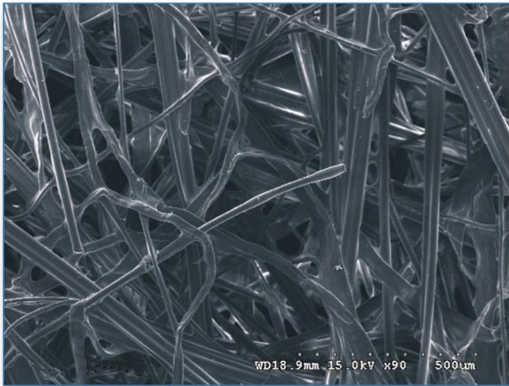
Figure 5-2 Scanning electron microscope image of a polyester-glass fiber filter
